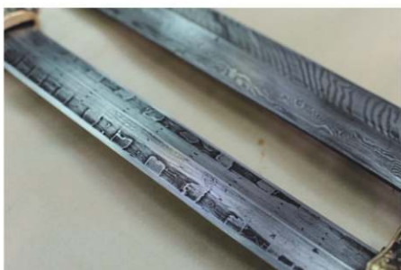
獨特劍紋展現極致鍛造技藝 Kuo has patented a multiple-layered veined steel manufacturing process.
